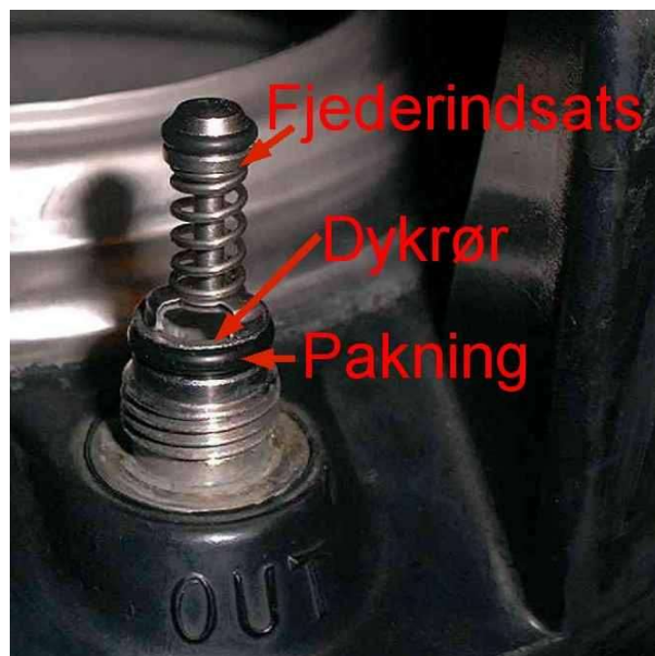
Fig. 10: Placering af dele i lynkobling.
